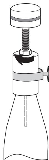
Turn the logger to the right into the bottle adapter, until desired submergence is reached.
