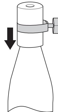
Turn the setscrew to the left, if the diameter of the clip is too small, in order to increase it. Push the adapter as far, as it rests shortly at the bottle neck.
