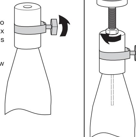
Turn the set screw to the right, in order to fix the adapter in this position.
